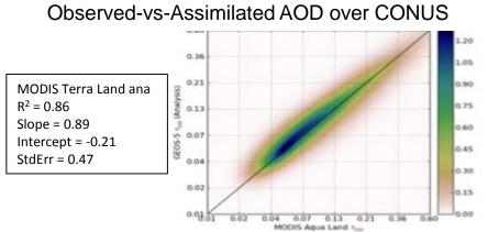
The performance of the aerosol assimilation system relative to satellite and aircraft measurements shows agreement between observed aerosol optical depth (AOD) from MODIS and the assimilation over land for the continental United States (CONUS).
