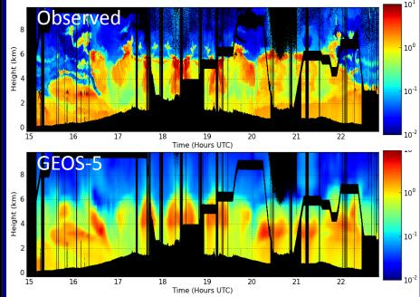
Aerosol backscatter observed (top) by the DIAL-HSRL instrument on NASA's DC8 and computed from the GEOS-5 aerosol analysis (bottom). The GEOS-5 data are sampled along the aircraft track.
