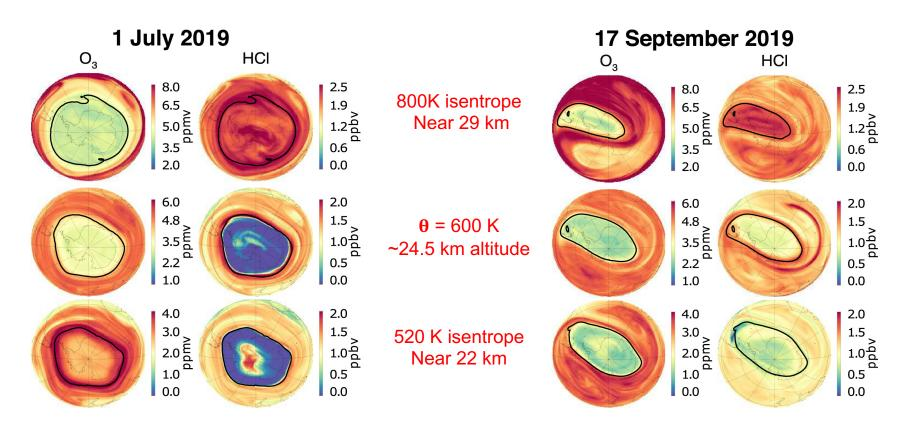
Large polar vortex (black contour). Chlorine activation indicated by very low concentrations of the chlorine reservoir compound, HCl at 600 K and below. No significant chemical ozone depletion yet. Smaller, distorted and displaced polar vortex following the sudden stratospheric warming. Low ozone. Increased HCI signals chlorine deactivation. Evidence of wave breaking.
