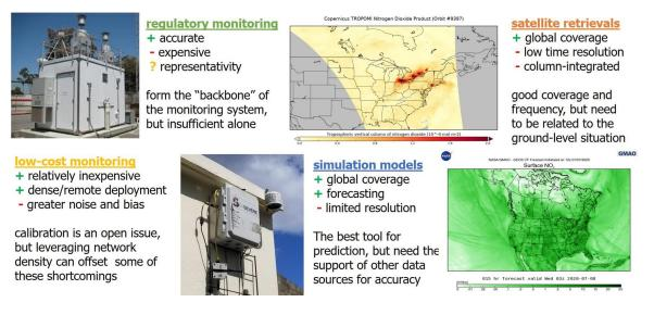
**Regulatory Monitors** form the baseline of air quality measurement data, with highly accurate and reliable instruments. However, as indicated above, these monitors are fairly sparsely deployed around the world, due to their high cost for purchase and operation. Their low density of deployment also leads to representativity issues, i.e., do the relatively few monitoring stations in an area fully capture the range of concentrations experienced by people living there?
